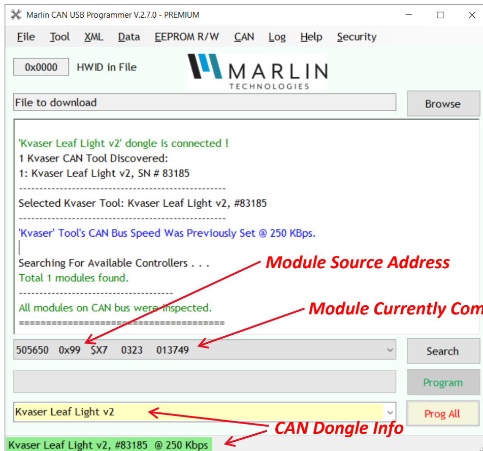
Figure 3: device being detected on the CAN bus. Shows CAN bus speed, source address and module information.
